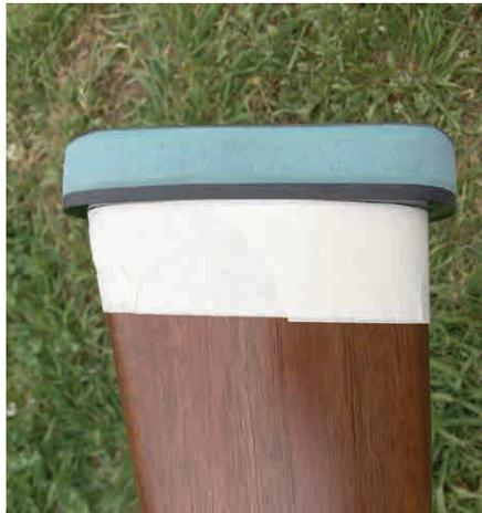
Masking tape applied before fitting.
